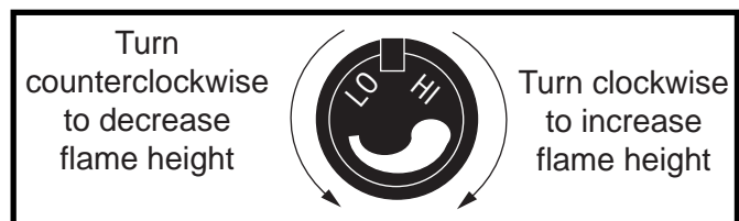
Fig. 59 Flame adjustment knob for Honeywell valve.
